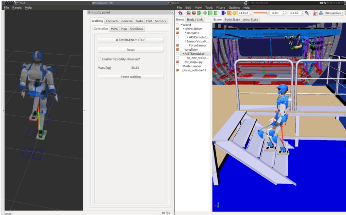
Controller with mc\_RTC GUI alongside a Choreonoid dynamic simulation
