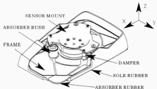
Fig. 18 Spring-damper mechanism of HRP-2 foot
