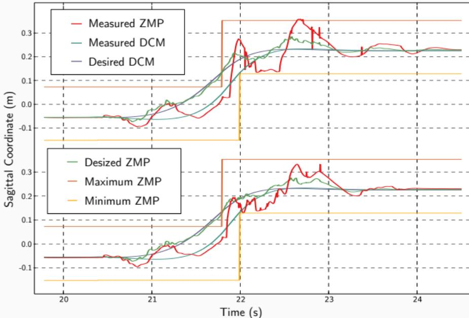
FIGURE 1: Top : no CoM admittance control. Bottom : with  $A_c = 20 \text{ [Hz}^2]$ .
