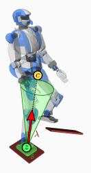
**Floating-base inverted pendulum (FIP)** Allow the ZMP to leave the contact area.<sup>1</sup>
