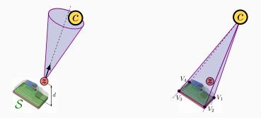
Figure 5: Friction constraint
