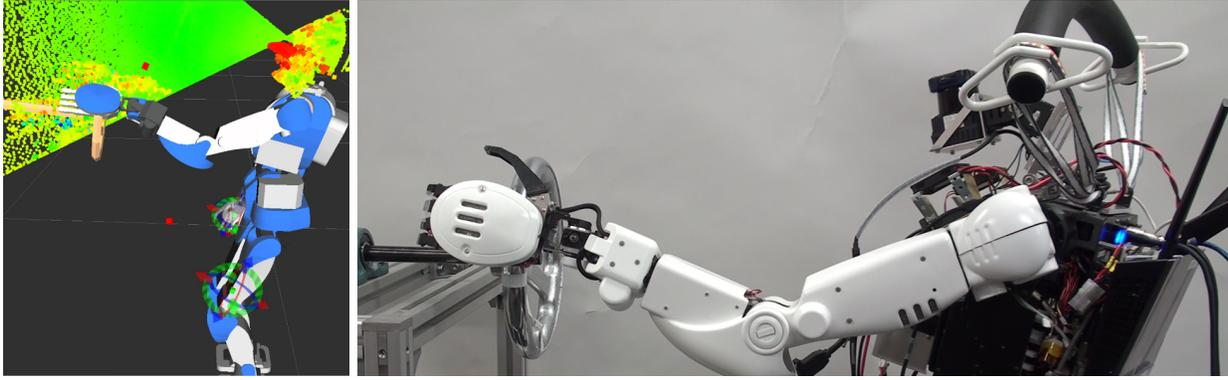
**Fig.2** Simultaneous view of the experiment in the OCS (left) and from a video camera (right). The Hokuyo laser-range sensor is mounted on top of a fixed plate set on top of the humanoid’s chest. Complete execution of the task took around 10 minutes to the human operator, including on-the-spot recovery of a loss of contact after three quarter-turns. See the accompanying video [2].
