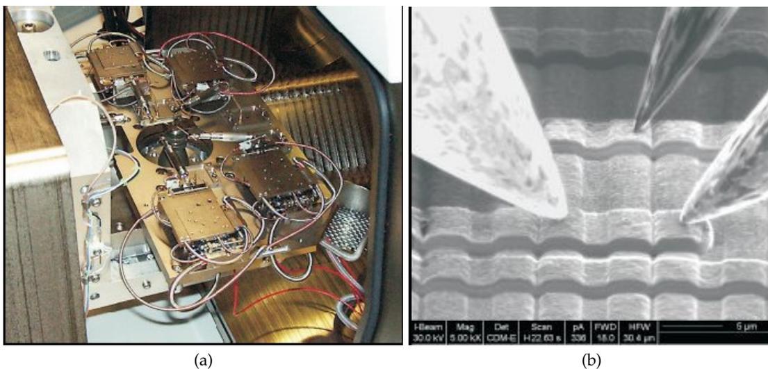
Fig. 23: A probing station mounted in a SEM and a tilted SEM view of circuit lines being probed.
